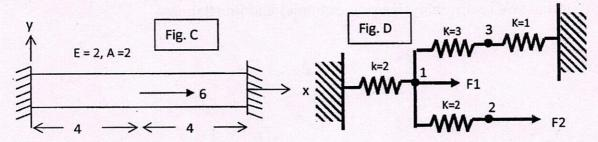
4. Solve the problem shown in the figure E for nodal displacement, element stress and reaction at the support. Take E = 100 GPa
