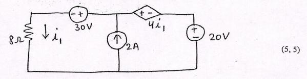
4. (a) Determine z-parameters of the network shown. An identical network is connected in series with this. Determine z-parameters for the overall network and verify the results by direct computation.
