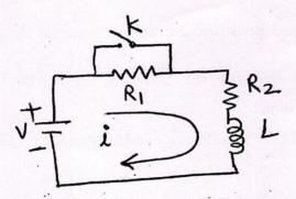
The switch k is closed at t=0, the steady state condition reached. Obtain the expression for the current in the circuit at time t. If  $R_1=R_2=100\Omega$ , V=10V and L=1H. Calculate at t=5 ms
