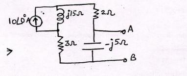
III. Determine Y and Z parameters for the networks shown as
