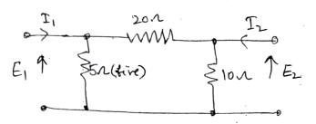
b) Calculate the z matrix of the two port network shown in the following figure
