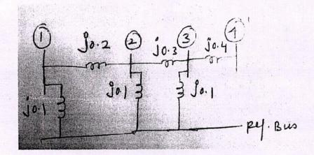
(b) The single line diagram of a three phase power system is as shown in Fig given below. The inductor to generator 3 neutral has reactance of 0.05 per unit using generator 3 ratings as a base. Draw zero, positive and negative sequence reactance diagrams using 1000 MVA, 765 kV base in the zone of line 1-2.
