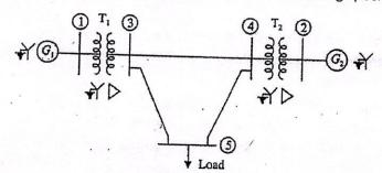
Generator  $G_1$ : 50-MVA, 1 1-kV, three-phase generator, X'' = 0.10 pu Generator  $G_2$ : 40-MVA, 6.6-kV, three-phase generator, X'' = 0.12 pu
