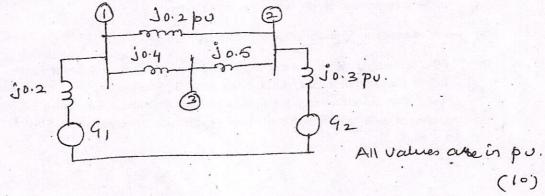
7. For the given network, find sub transient current in per unit from generator 1 and in line1-2, and the voltages at buses 1 and 3 for a three phase fault on bus 2 is 1.0 per unit with angle 0°.
