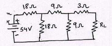
Determine the current flowing through R<sub>L</sub> when the value of load resistant is
