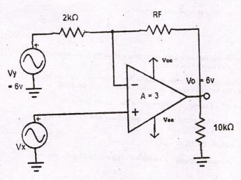
(j) From the circuit, determine the output voltage (Assume  $\alpha_r$ =1)
