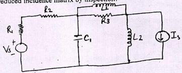
b) Determine the transmission parameters for the network shown below.
