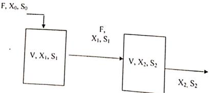
6. A) A feed solution containing a enzyme A ( $C_A = 1 \text{ kmolm}^{-3}$ ) is fed to a CSTR or to a PFR at a reaction rate constant is  $0.02 \text{ s}^{-1}$ , and converted to product P in the reactor. The first-order to attain a fractional conversion of A,  $X_A = 0.95$ .
