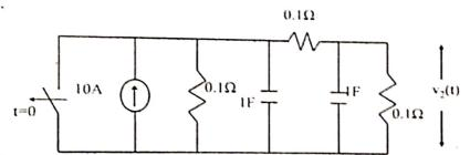
Find the power loss in the resistors of the network shown below using nodal (b) (5) analysis.
