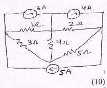
IV. Determine transmission parameters of the network shown using concept of intersection of 2 two-port networks in cascade:
